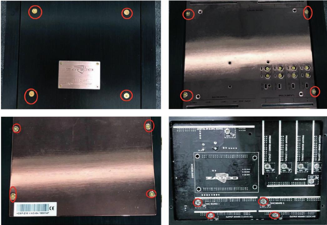
4. Remove the OMAP module, DAC boards and OUTPUT boards.
