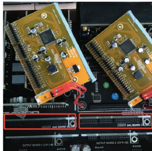
8. Install the DAC boards into the sockets and it should look as shown (on the left). Also shown SOCKET for OUTPUT BOARD (on the right).
