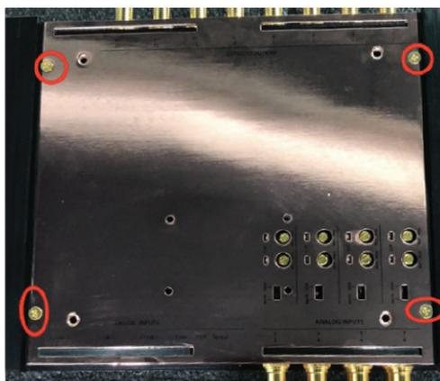
Notes: Pay attention the direction /position of OMAP module. If the screws can't be tighten that means DAC or OUTPUT boards are not in the right position. The length of the wires can be adjusted for a better installation.
