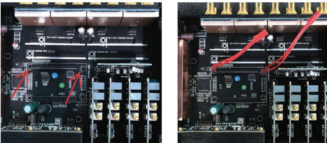
6. Solder the wires to +5V\_D at the points shown. Then turn the Unit over and prepare it for assembly with the new DAC (or DACs) and Output Board (or Boards).
