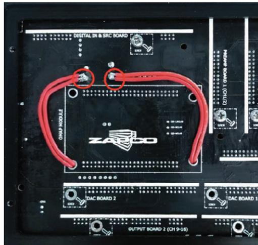
7. Connect the wire harnesses to the DAC boards (16-Ch. processor shown).
