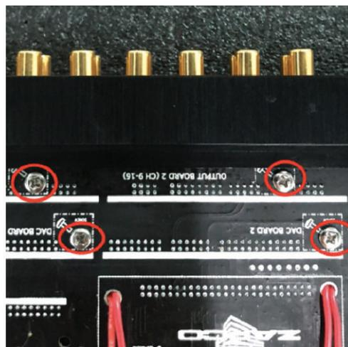
11. Tighten screws of the bottom panel. Put back the top under cover and tighten the screws.
