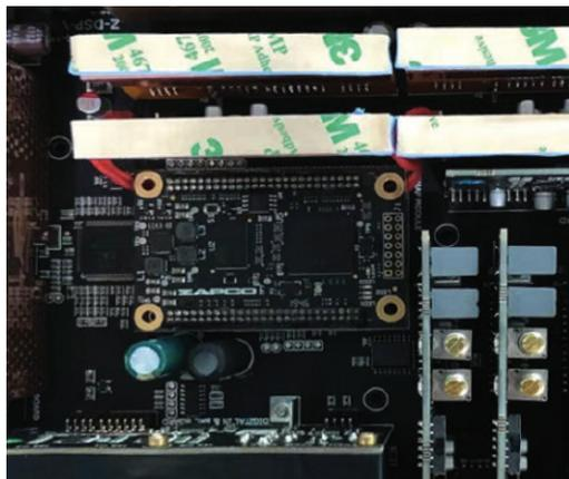
10. Tighten the screws for DAC boards and OUTPUT boards, after screws are tightened please use force to press boards to make sure that they are inserted into sockets well, if screws do not thread easily then the boards are likely not in correctly and should be rechecked.
